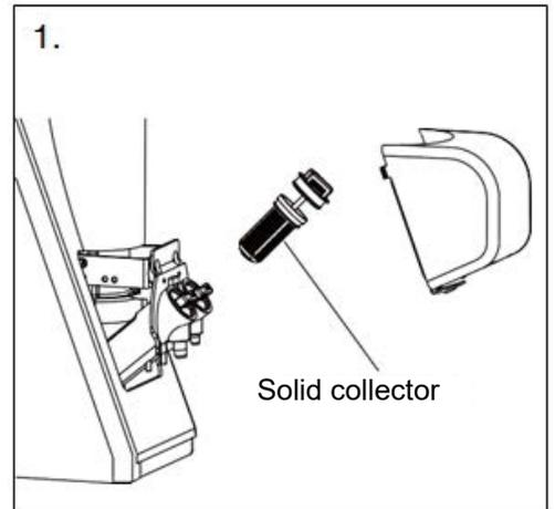
To remove the filter from the solid's collector, push the bar from the front side of the collector and clean the filter with running water.
