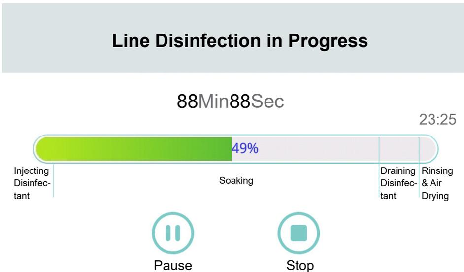
The system can be paused or stopped at any time during operation.
