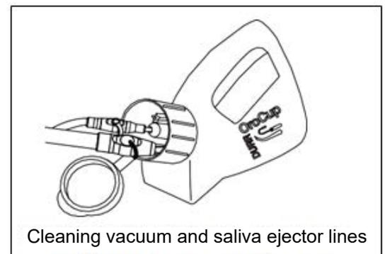
Cleaning vacuum and saliva ejector lines
