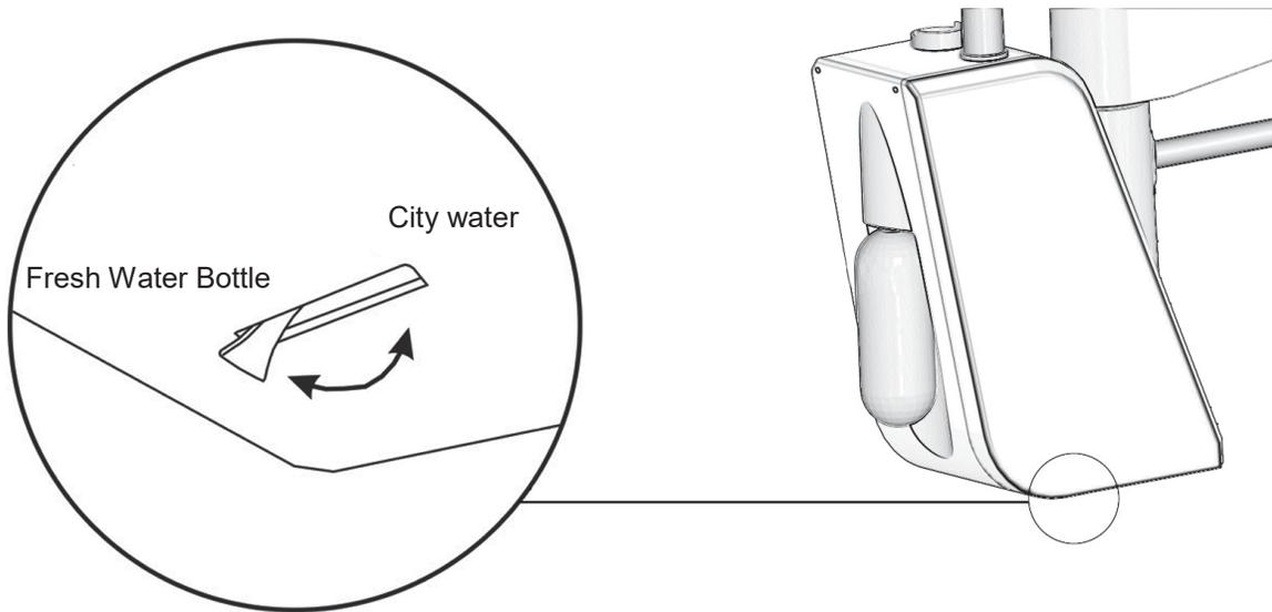
The user can switch between city water and distilled water
