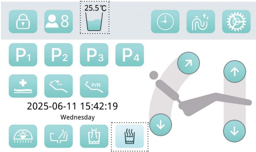
When the system is equipped with a heater and the heater is in the on position,
