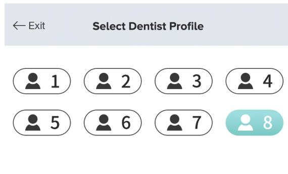
When the system is powered on, it will automatically select the Dentist profile from before the system was shut down.
